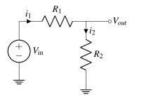
$$\begin{split} i_2 &= \frac{V_{out}}{R_2}, \ i_1 = \frac{V_{in} - V_{out}}{R_1} \\ i_1 &= i_2 \\ \frac{V_{in} - V_{out}}{R_1} &= \frac{V_{out}}{R_2} \\ \frac{V_{in}}{R_1} &= V_{out}(\frac{1}{R_1} + \frac{1}{R_2}) = V_{out}(\frac{R_1 + R_2}{R_1 R_2}) \\ V_{out} &= \frac{R_2}{R_1 + R_2} V_{in} \end{split}$$
