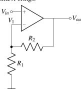
$$V_{out} = A(V_{in} - V_1), V_1 = \frac{R_1}{R_1 + R_2} V_{out}$$
