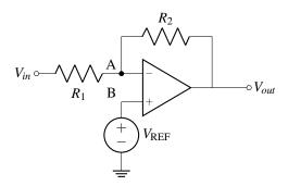
From the first golden rule, we know the fact that node B is at  $V_{REF}$  means that node A is as well. From the second, we have the equation
