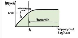
$$V_{\text{out}}^{N} = V_{\text{in}}^{N} \cdot \frac{Z_{R}}{Z_{R} + Z_{c}} = V_{\text{in}}^{N} \cdot \frac{R}{\frac{1}{jwc} + R}$$
