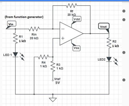
Inverting amplifier, but with an offset No current into inputs of op amp, so
